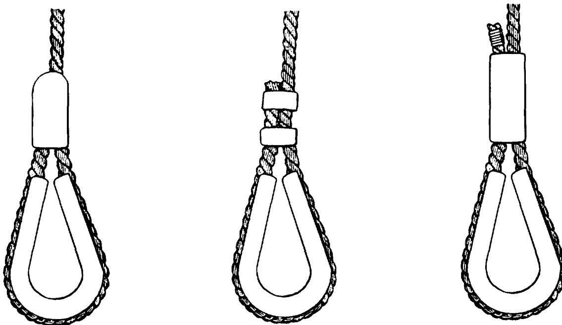
Figure 3-33.—Fold back eye and pressed metal sleeve.
